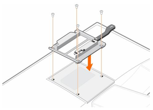
Attaching the Client —Slightly tip the client to align and insert the four protruding shoulder screws into the four cutout areas of the E series mount. Slide the client until it clicks and secured by latch. The security latch will move automatically when the shoulder
